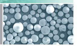
Used as industrial column packing material for general purification of natural products, food, cosmetics as well as in pre-purification of pharmaceutical and nutraceutical ingredients. ZEObeads are preferably used in liquid chromatography, flash chromatography and solid phase extraction.
